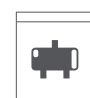
Splitter If connecting multiple devices to one cable wall outlet, you will need to use a splitter
